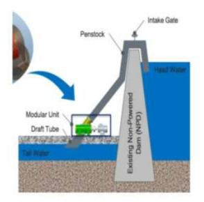
Fig. 3: Powering of Non Powered Dams
